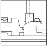
This has a mating ring annulus around the outside diameter (OD and is used in conjunction with a chamfered mating ring to direc flow at the sealing faces.
