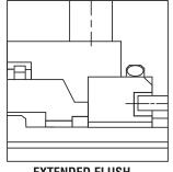
This is a single point injection, providing maximum exposure of the mating ring surface.
